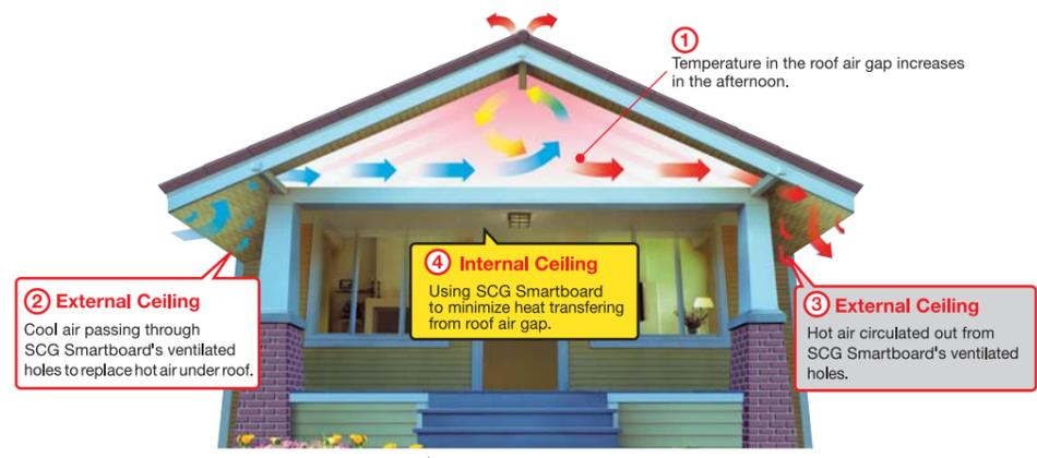
**SCG Ventilation Ceiling System** enables energy efficiency with living comfort. **SCG Smartboard Ventilation** series helps circulate air flow under the roofing with the factory-made drilled holes suitable for external eaves ceiling application guaranteed moisture and water resistance.
